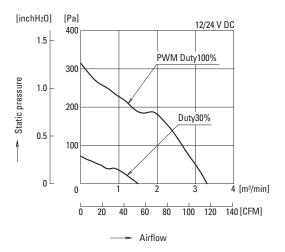
Fig. 6: 92 mm sq. 38 mm thick "San Ace 92T" airflow vs. static pressure characteristics
