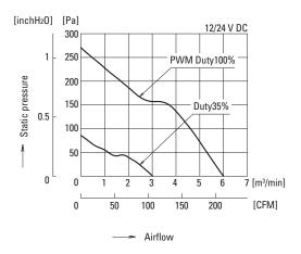
Fig. 7: 120 mm sq. 38 mm thick "San Ace 120T" airflow vs. static pressure characteristics
