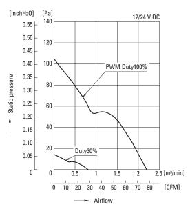
Fig. 5: 92 mm sq. 25 mm thick "San Ace 92T" airflow vs. static pressure characteristics
